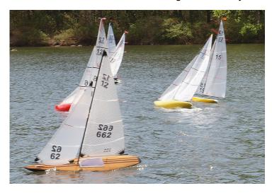
can see from the pictures, the size of the boats are ideal for getting that "real" feeling for sailing. The EC-12 is a restricted one design radio controlled model yacht class with fiberglass hulls made from near identical molds and otherwise restricted to similar construction. The result is a class of boats with
